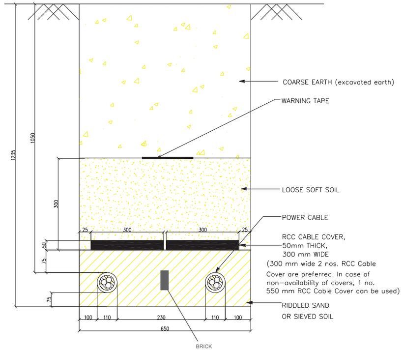
**Figure 1.6 – 33kV Buried Cable for Double Circuit**
