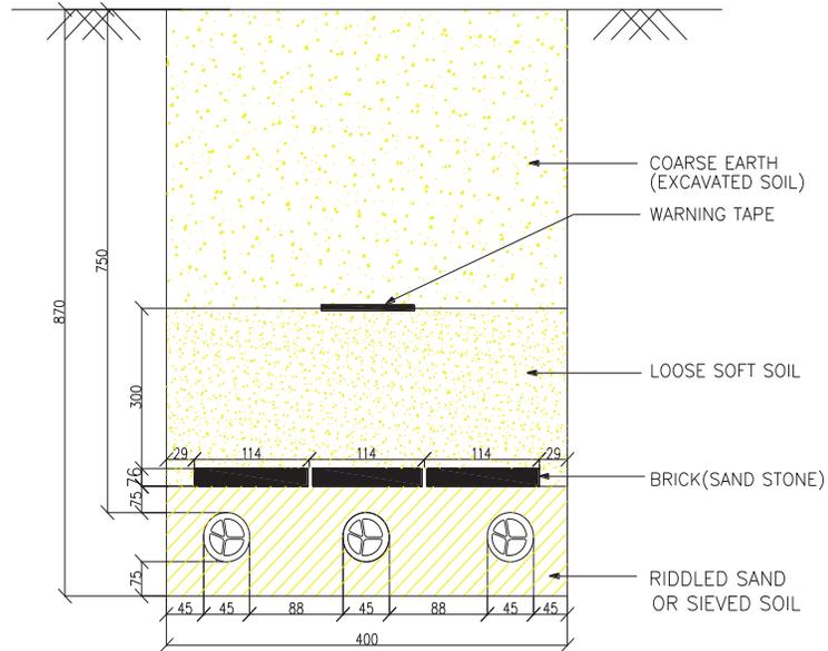
**Figure 1.1 – 1.1kV, 150sqmm Buried Cable**
