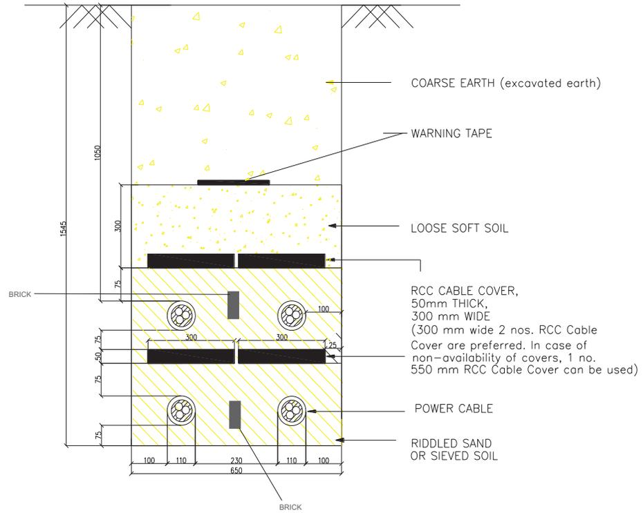
**Figure 1.7 – 33kV Buried Cable Option-1 for Four Circuits**
