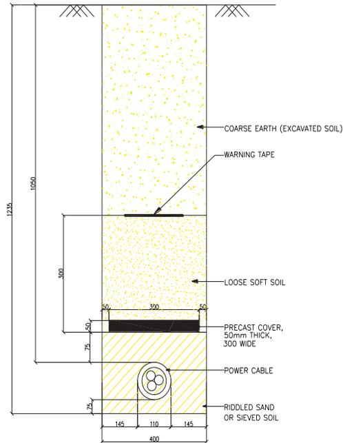
**Figure 1.5 – 33kV Buried Cable for Single Circuit**
