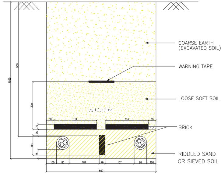
**Figure 1.4 – 11kV Buried Cable for Double Circuit**
