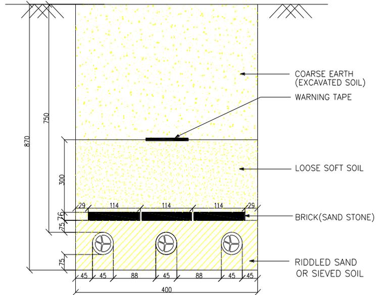
**Figure 1.1 – 1.1kV, 150sqmm Buried Cable**
