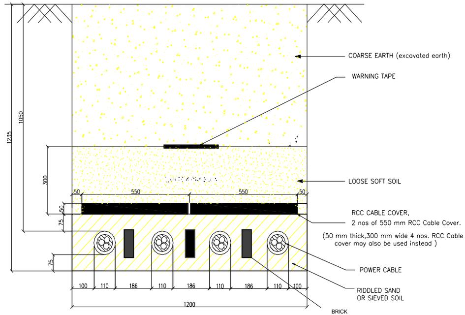
**Figure 1.8 – 33kV Buried Cable Option-2 for Four Circuits**
