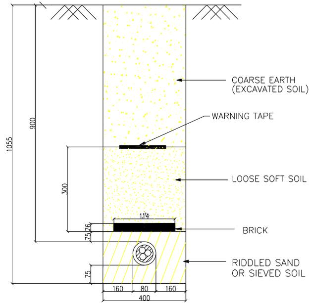
**Figure 1.3 – 11kV Buried Cable for Single Circuit**
