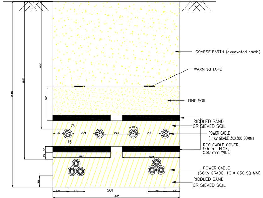
**Figure 1.10 – 66kV Double Circuit and 11kV Circuits**
