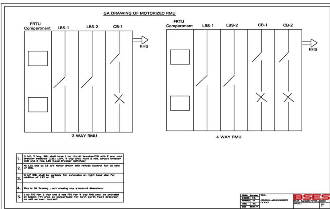
a) 11kV RMU shall have circuit breakers (CB) with Load break switches (LBS) as per configuration defined in Purchase Requisition.
